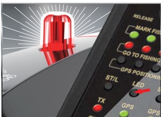
Press the "LED" button one time, the night navigation light turns on, press the button again, the night navigation light turns off.
