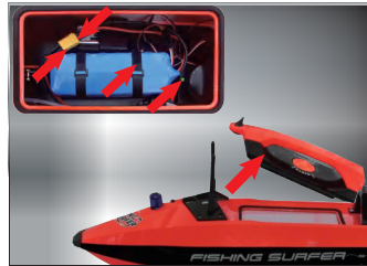
Put battery inside, fix it with velcro strap. Use battery plug to plug in receiver power connector, the light on the receiver turns on ( remarks: The transmitter shall switch on before receiver switch on), then the control system is working.
